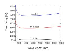
Maximum delay relative to the asymmetric (ASY) configuration achievable with the three different models (S, M and L) as a function of wavelength.
