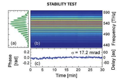
(a) Fringe pattern generated by the interference of the two replicas created by the GEMINI 2D Interferomter; (b) sequence of fringe patterns acquired by keeping the relative delay fixed for 30 min; and (c) corresponding phase fluctuations. The phase jitter is less than 1/360th of the optical cycle.
