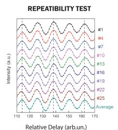
Interference patterns between the two replicas generated by the GEMINI 2D Interferometer, measured for different scan number indicated on the right. The lower one is the average of 40 scans. The measurements show an exceptional repeatibility!
